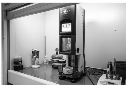
FEI Vitrobot Mark IV: Vitrification device for sample preparation for cryo-electron microscopy
