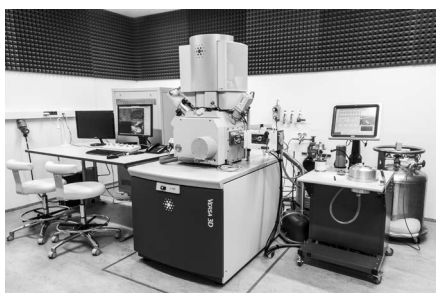
FEI Versa 3D FIB/SEM microscope. Small dual-beam microscope for preparation of thin cellular sections from vitrified material equipped with cryo-stage and device for sample transfer under cryo-conditions.
