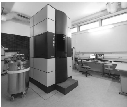
FEI Titan Krios microscope: High-end transmission electron microscope for cryo-electron microscopy equipped with direct electron detector camera Falcon2.
