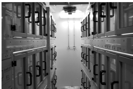
Cultivation banks serve for precisely controlled plant cultivation and comparison studies.
