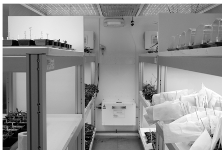
Walk-in plant growth chamber (FytoScope, PSI) that utilizes LEDs as a sole light source.
