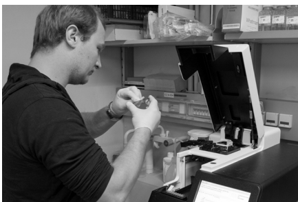
Loading a cBot clustering system
