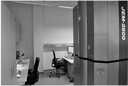
Scanning Transmission Electron Microscope: Joel JEM2800 + 3D Tomography + EDS system
